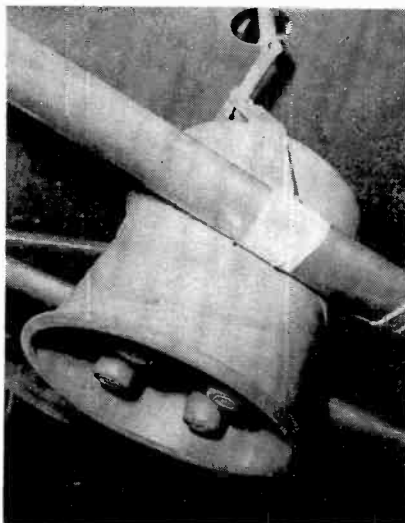
▲ Something new in plane PA installations. Two University 4-unit speakers fit close under wing, hung from 4-point mountings; ← two side straps anchor on struts, and two rings on overhead bar, welded to plane's frame.
