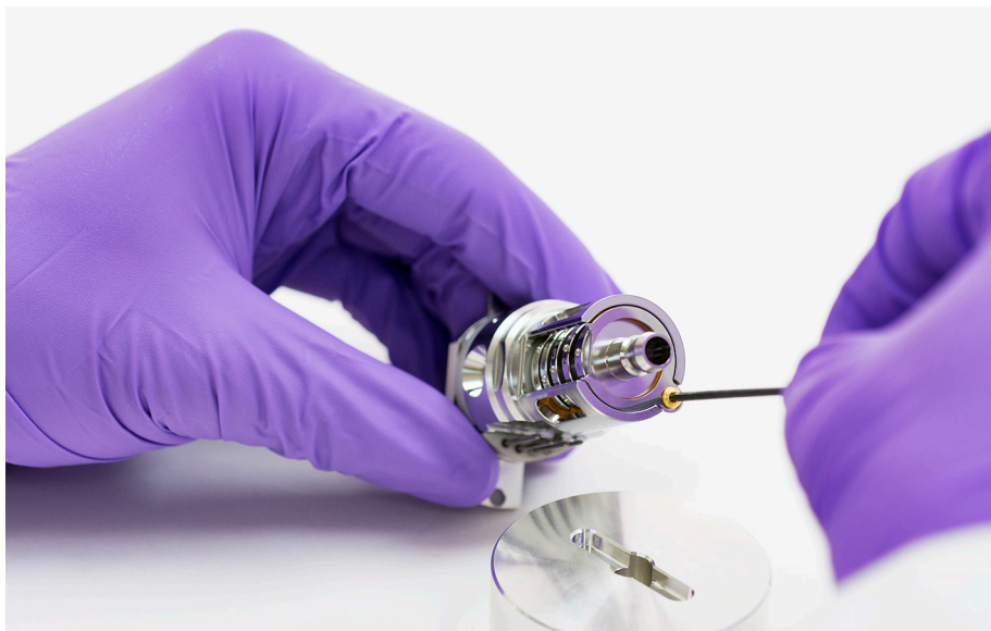
Figure 23. Secure the lens screw and lock ring insulator
