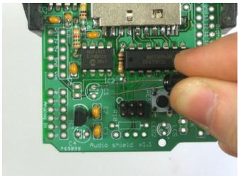
Next are the three electrolytic capacitors C1 C4 and C9.
