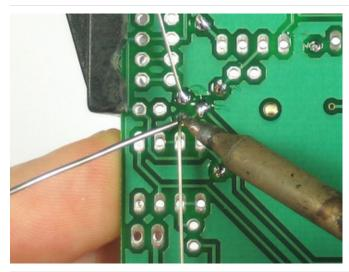
Solder and clip the small capacitor leads.
