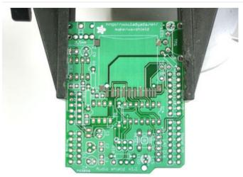
Get ready by placing the PCB in a vise.
