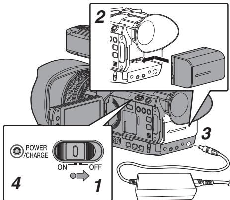
1 Hold down the lock button (blue) at the center of the [POWER ON/OFF] switch to set to "OFF".
