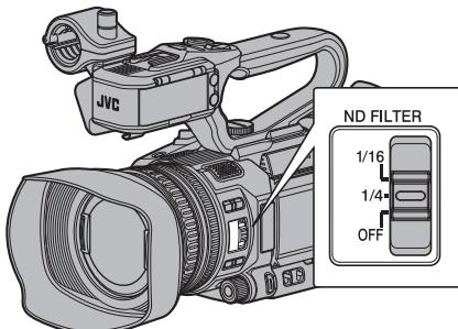
Switch according to the brightness of the object. When the position on the switch is changed, the selected position of the ND filter is displayed on the LCD monitor and viewfinder screen.
