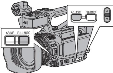
To set only the Gain, Iris and Shutter to Auto mode, press and hold the [FULL AUTO] button and set the Full Auto mode to off before setting each item to the automatic adjustment mode.
