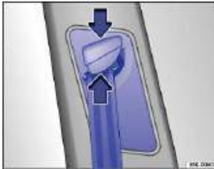
Fig. 67 Next to the front seats: Safety belt height adjuster.
