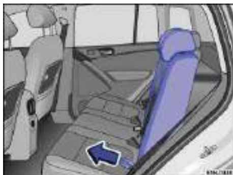
Fig. 45 Adjusting the rear backrest.
