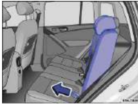
Fig. 97 Folding the backrest forward and back.
