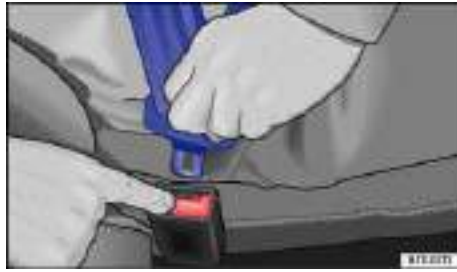
Fig. 64 Releasing the buckle tongue from the belt buckle.
