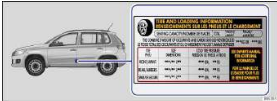
Fig. 112 Location of the tire inflation pressure label.
