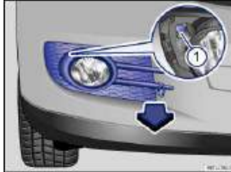
Fig. 202 In right front bumper: Removing light assembly.
