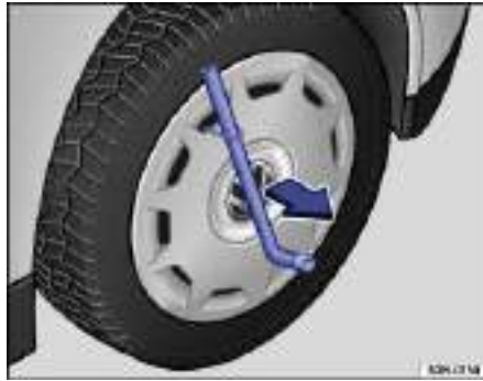
Fig. 190 Pulling the wheel cover off.
