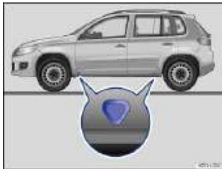
Fig. 192 Lift points for the jack.
