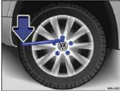
Fig. 191 Changing a wheel: Loosening wheel bolts.
