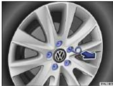
Fig. 189 Pulling cover caps off wheel bolts.
