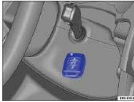
Fig. 136 Emergency starting feature on vehicles with Keyless Access.
