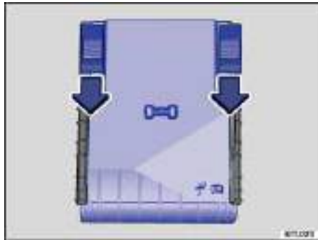
Fig. 197 In the engine compartment: Fuse box cover.
