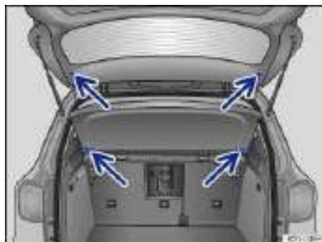
Fig. 100 Installing and removing the luggage compartment cover.
