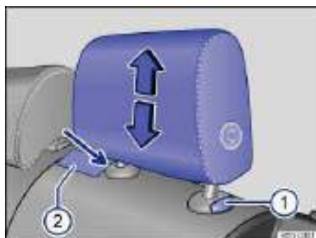
Fig. 49 Removing the rear head restraints.
