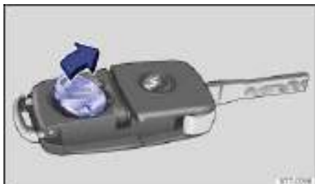
Fig. 24 Remote control vehicle key: Remove old battery.
