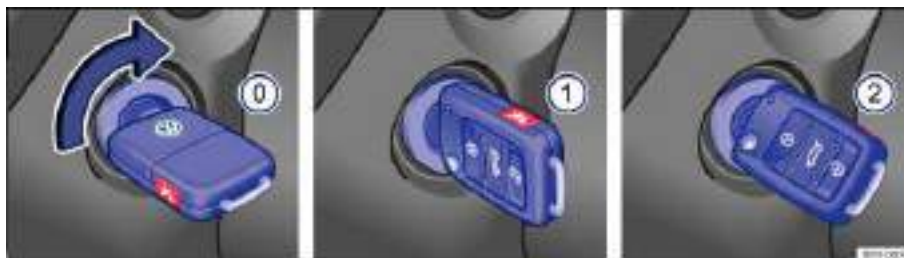
Fig. 134 In the ignition switch: Vehicle key positions.
