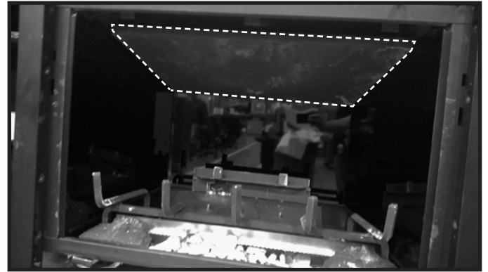
Figure 4. Install Top Refractory Panel
