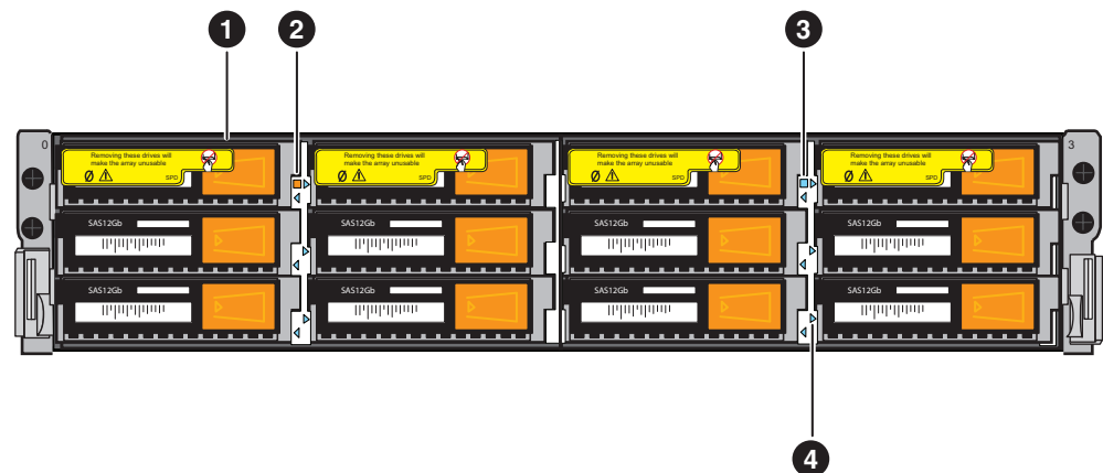
Figure 3 Example of the 2U, 12 (3.5-inch) disk drive DPE (front view)
