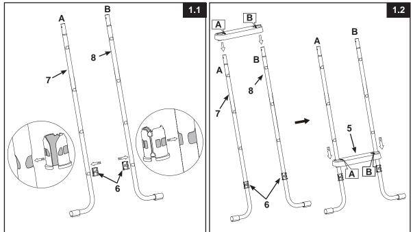
**IMPORTANT:** Ensure the J-shaped legs are pointing outwards before installing the steps.
