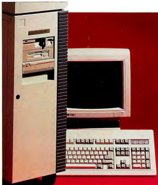
The CCS 486-25c EISA features a Mylex MAE486-25 motherboard with a Phoenix BIOS. Its 128K bytes of write-back cache provides zero-wait-state operation.
