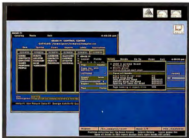
dBASE IV for Sun includes the dBASE IV Control Center, from which you access the program's design tools and code generator.
