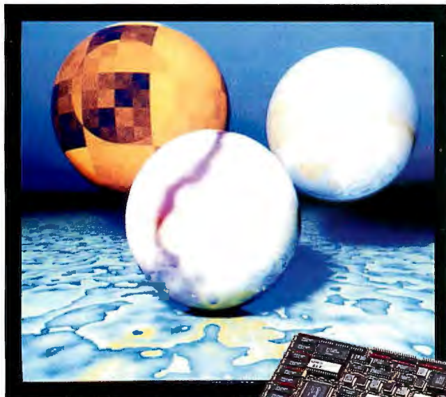
Photo 1: Monolithic's MicroPaq 452 Ultra uses a custom graphics chip from Edsun Labs to simultaneously display 700,000 colors on a standard VGA monitor.
