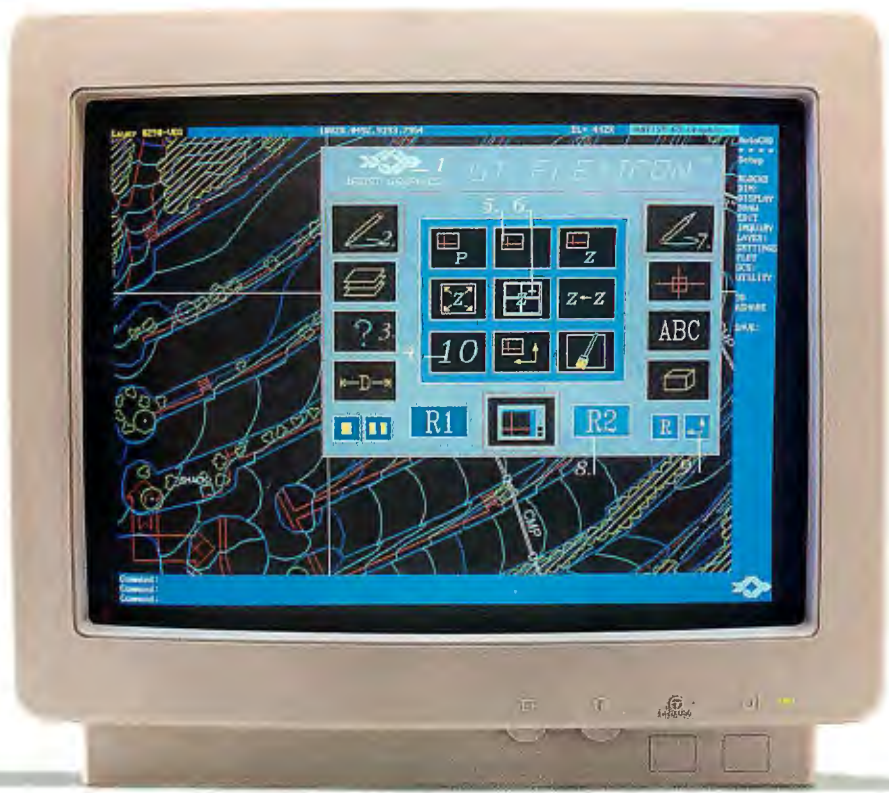
1. Help Icon 2. AutoCAD Sub-Menu Icon 3. Icons Are Made In AutoCAD 4. GT Top 10™ 5. Bird's-Eye Icon 6. GT Flexicon Pops Up At Cursor 7. Hot Spots to Nested Sub-Menus 8. Reassignable Icon 9. Resize Icon
