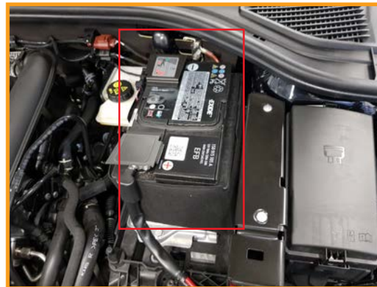
12V Battery in the Engine Compartment
