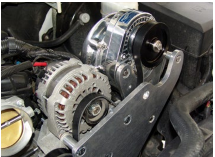
Sub-Bracket Assembly Installed
