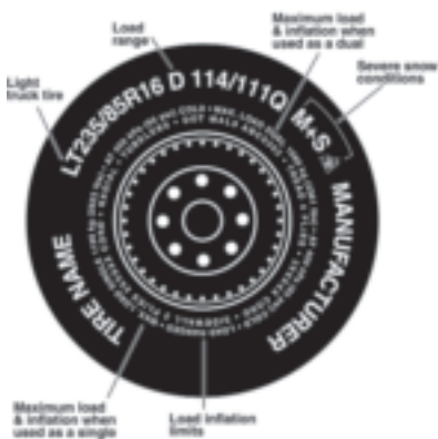
Figure 4: Typical Light Truck Tire Markings
