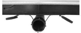
Black/Grey Tank Drain and Valves
