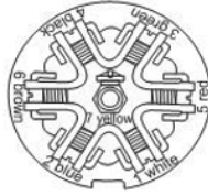
7-way trailer plug car end, rear view
