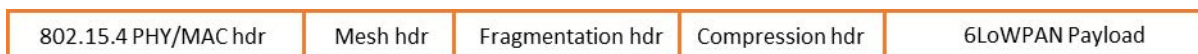
Figure 3.4. 6LoWPAN Packet Containing Mesh Header, a Fragmentation Header, and a Compression Header
