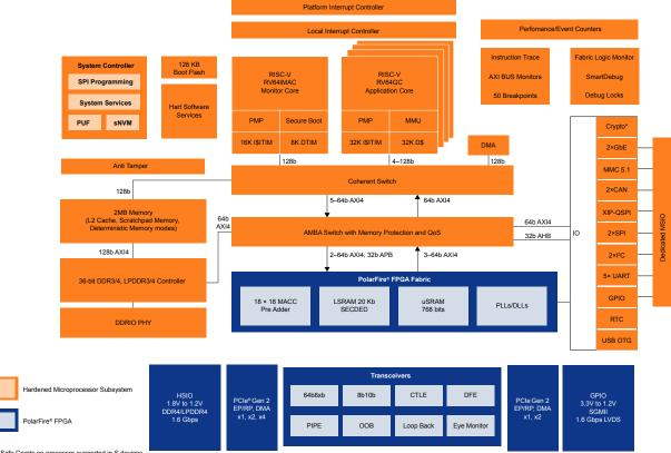
\*DPA-Safe Crypto co-processor supported in S devices \*\*SECDED supported on all MSS memories
