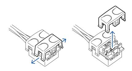
4. Remove the 2 caps from the top of the Controller's connector. Pull up on the tabs to relase the caps.
