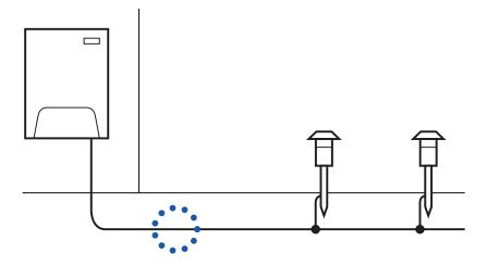
2. Locate the low-voltage wire that runs between your transformer and the first of the landscape lights. Choose a place along the wire in the lawn or landscaping, where the Controller's stake can be inserted into the ground. Here, the Connector will attach to the low-voltage wire.
