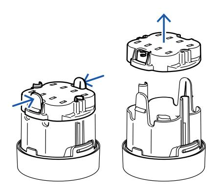
2. Press and squeeze the top and bottom tabs of the compartment cover to open it.
