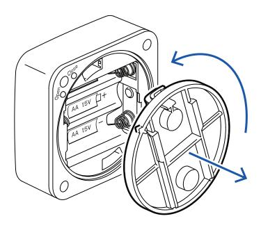
1. Press your palm against the rear plate and twist counterclockwise (about 5°) to open and access the battery compartment.
