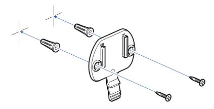
3. Fix the mount to the wall with screws. Use anchors if needed.
