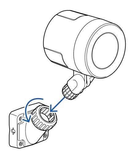
2. Twist the locking-ring on the wall mount to loosen it, and insert the base of the Spotlight.
