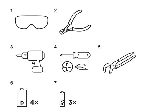
1 protective eyewear 2 wire stripper / cutter (18 to 12 gauge wire)
