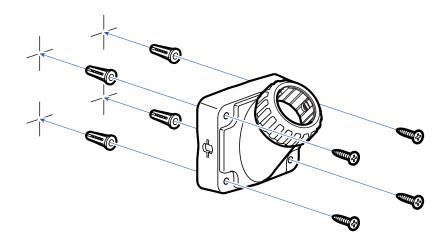
1. Choose a location on the wall 4 to 6 ft. above the ground to mount the Spotlight. Fasten the mount to the wall. Use anchors if needed.
