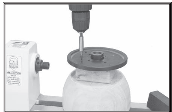
Figure 35. Example of mounting workpiece to a faceplate using a backing block.
