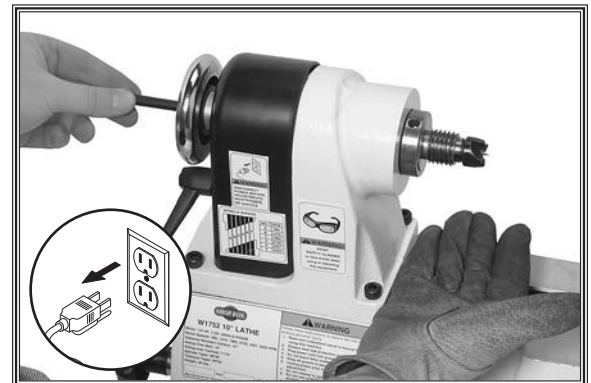
Figure 23. Example of removing spur center using knock-out bar.
