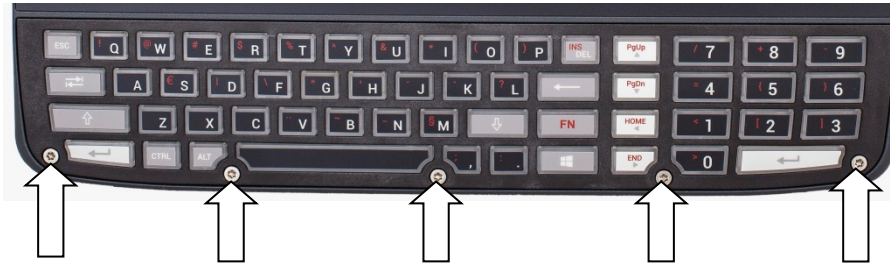
Fig. 13.1: Unscrew the mounting screws of the integrated keyboard
