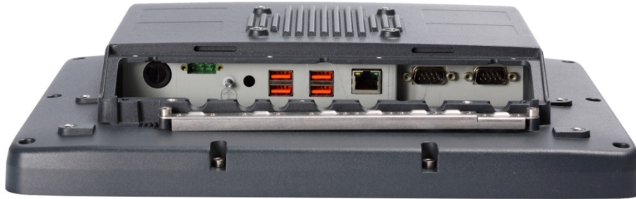
Fig. 9.1: External connectors under the cable cover
