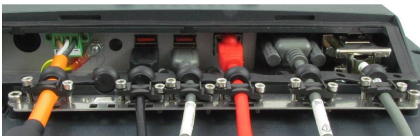
Fig. 8.7: COM cable on the connector panel; secured to the strain relief rail
