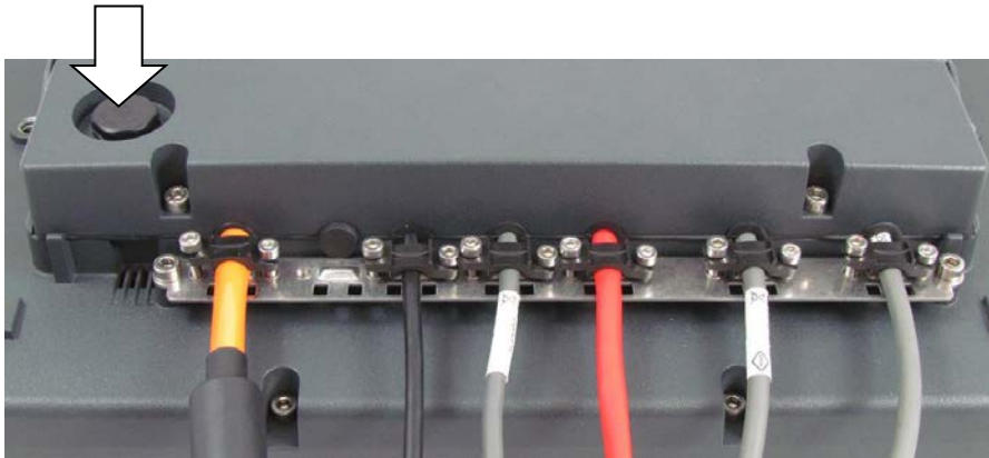
Fig. 8.10: Pressure compensation element - Do not modify or remove
