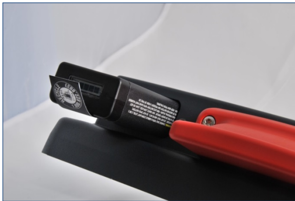
Fig. 12.2: Inserting the battery pack in the battery pocket
