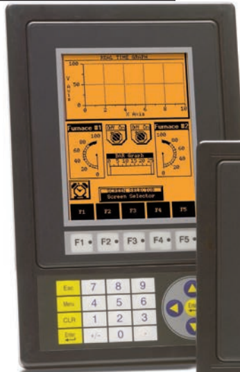
C-more 6" Micro-Graphic Panel Installed in a 21-button Portrait Keypad Bezel EA-MG6-BZ2P
