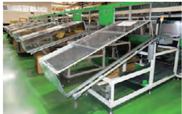
Automated toner cartridge sorting system
