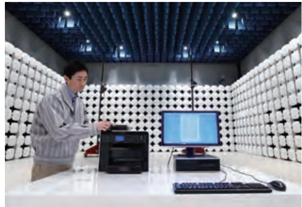
EMI measurement of products in an anechoic chamber
