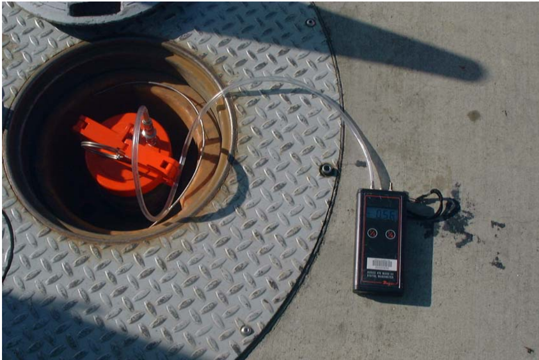
Figure 8-2 - Typical Field Installation of UST Pressure Measurement Assembly
