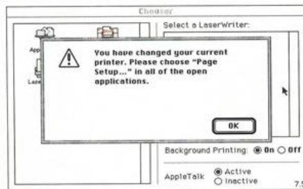
Not all printing problems are to do with fonts. If you change your printer you must tell all your applications, for instance.
