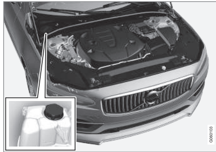
Coolant expansion tank, left-hand drive vehicle
