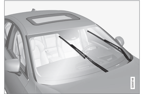
Windshield wipers in the service position.
