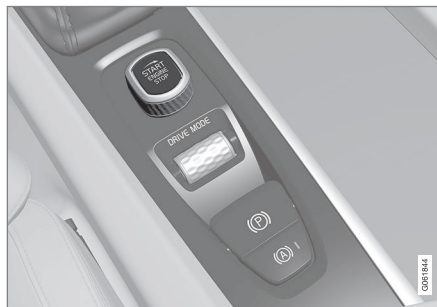
Start knob in the tunnel console.
