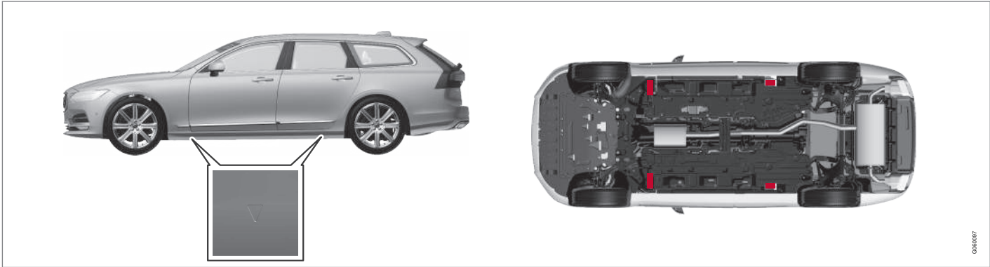
The triangles in the plastic covering indicate where the jack attachment points/lifting points (red areas) are located.
