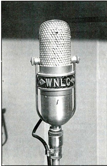
An RCA DX-77 ribbon mic with a rare WNLG center "flag" ring. It hails from the 1490-kc era.
