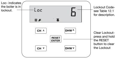
Figure 12.1: Lockout Display Screen
