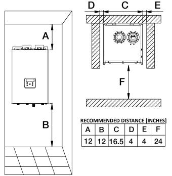
Figure 3.2 - Minimum Installation Clearances
