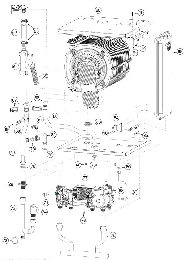
Figure 15.2: Cabinet Interior Wet Side Parts
