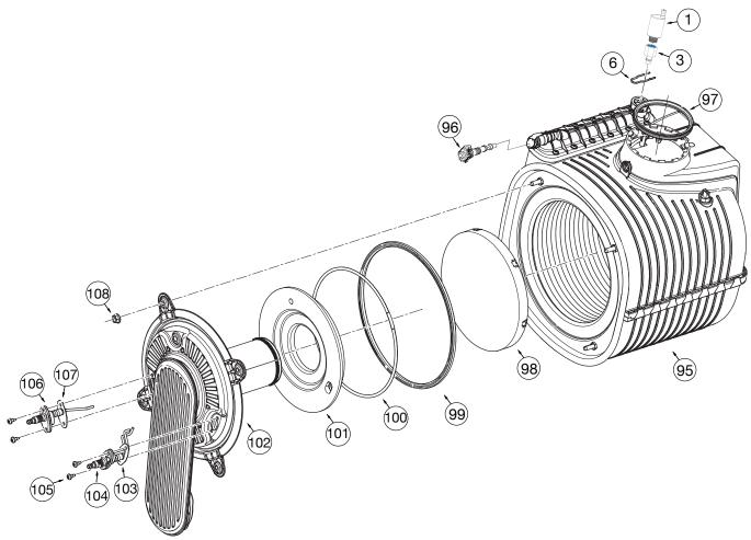
Figure 15.5: Heat Exchanger Parts
