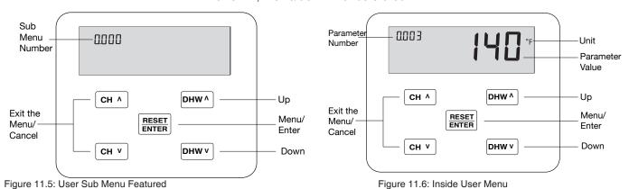
Param. Value Description # 0.003 CH setpoint Temperature 0.048 DHW setpoint Temperature 0.200 System Test Menu (visible only after input of Installer code) °C/°F 0.901 Temperature unit setting 0.902 Pressure unit setting bar / psi
