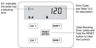
Figure 12.2: Blocking Error Display Screen
