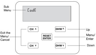
Figure 11.9: Main Menu Screen with CodE Menu Highlighted
