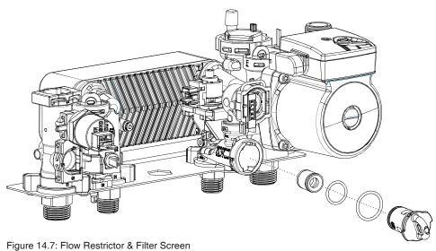
Figure 14.7: Flow Restrictor & Filter Screen
