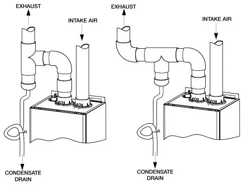
Fig 4.1: Vertical Drain Tee with Trap
