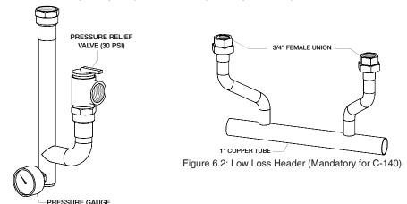
Figure 6.1: Pressure Relief Assembly
