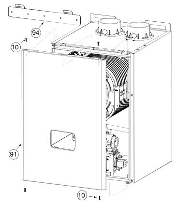
Figure 15.4: Front door Assembly
