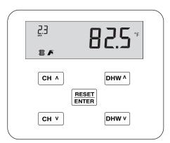
Figure 11.4: Main Screen in standby mode.
