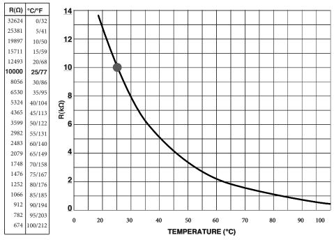
Table 12.3: Sensor Resistance Value Versus Temperature
