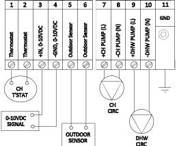
Figure 9.1: Simplified Wire Connections
