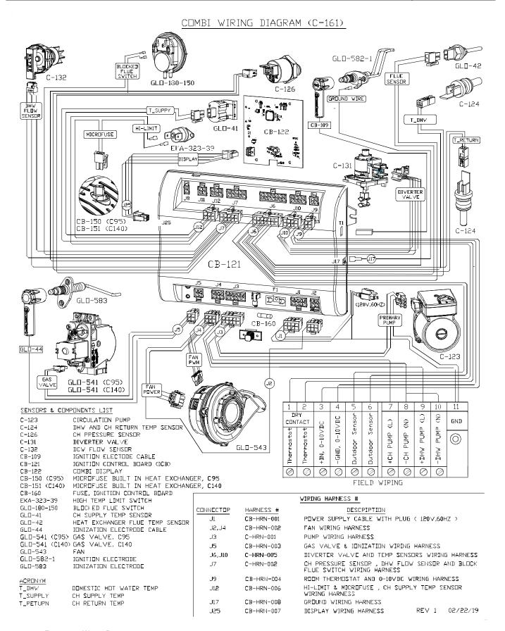
Figure 9.3: Wiring Diagram
