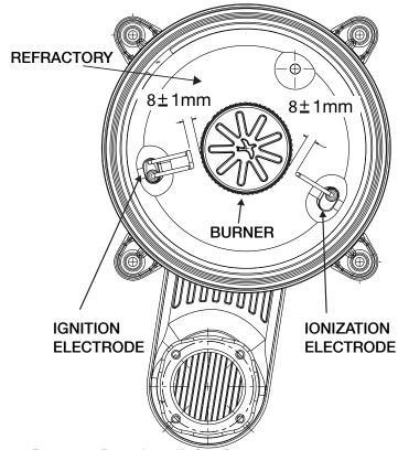
Figure 14.5: Burner Assembly Specifications
