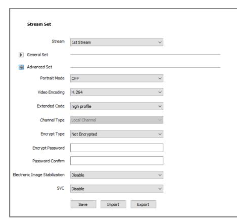
Under the **Advanced Set** section, you select video encoding (H264, H265, MotionJPEG), extended code (If H.264 is selected, choose high profile, main profile, or baseline), channel type (fixed to local for cameras), encryption type (that is, whether or not to require a password) and password, electronic image stabilization, and SVC (scalable video coding).
