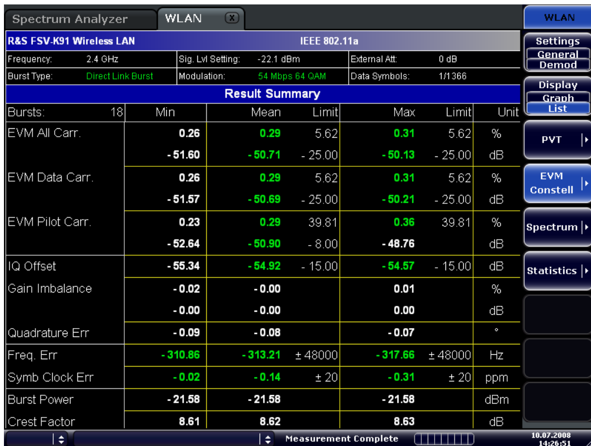
Figure 3-13: Result summary list for measurements on OFDM signals
