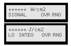
'OVR RNG': This message will blink in the 'status' register (lower right corner of the LCD) when the input detector signal exceeds the measurement range of the system. In addition, plus signs take the place of numerals i n the data display, so that the top line will read '+++++ W/
