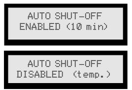
'ZERO' button: To advance the 'MENU' to screen # 3. 'INTEGRATE' button: To 'INCREMENT' the bottom line between three choices: 'ENABLED (10 min)', 'DISABLED (temp.)', and 'DISABLED (PERM.)'.
