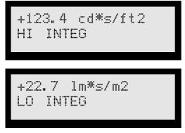
'HI INTEG' or 'LO INTEG': One of these messages is displayed continuously in the 'mode of operation' register (lower left corner of the LCD) after the 'INTEGRATE' button has been pressed, indicating that the instrument is in light integration mode. Press the 'INTEGRATE' button twice within one second to alternate between the 'HI' and 'LO' integration ranges. Press the integrate button once t o reset the integral register in that mode to zero.
