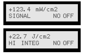
'NO OFF': This message will blink in the 'status' register (lower right corner of the LCD) when the automati c 10 minute shutoff feature has been disabled. This indicates that a previous user selected 'AUTO SHUT OFF' 'DISABLED' using the programming mode capabilities.
