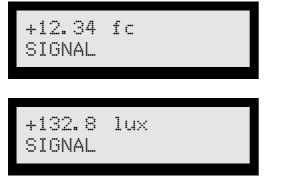
'SIGNAL': This message is displayed continuously in the 'mode of operation' register (lower left corner of the LCD) after the 'SIGNAL' button has been pressed, indicating that the instrument is in constant wave measurement mode.
