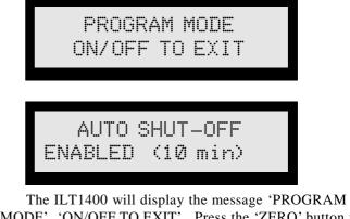
The ILT1400 will display the message 'PROGRAM MODE', 'ON/OFF TO EXIT'. Press the 'ZERO' button to select the 'AUTO SHUT-OFF' menu. The 'ZERO' button selects through the numerous changeable 'MENU' screens.
