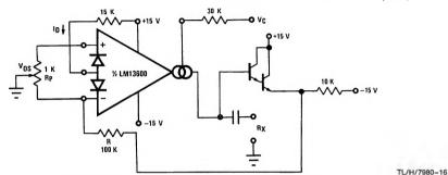
FIGURE 9. Voltage Controlled Resistor with Linearizing Diodes
