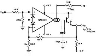
FIGURE 11. Voltage Controlled Low-Pass Filter
