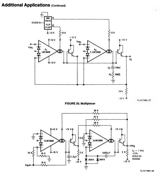
FIGURE 21. Phase Lock Loop
