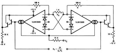
FIGURE 10. Floating Voltage Controlled Resistor
