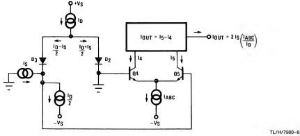
**FIGURE 1. Linearizing Diodes**
