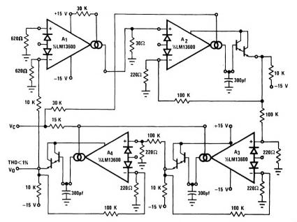
FIGURE 17. Sinusoidal VCO
