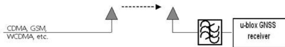
Figure 18: Measures against out-of-band interference
