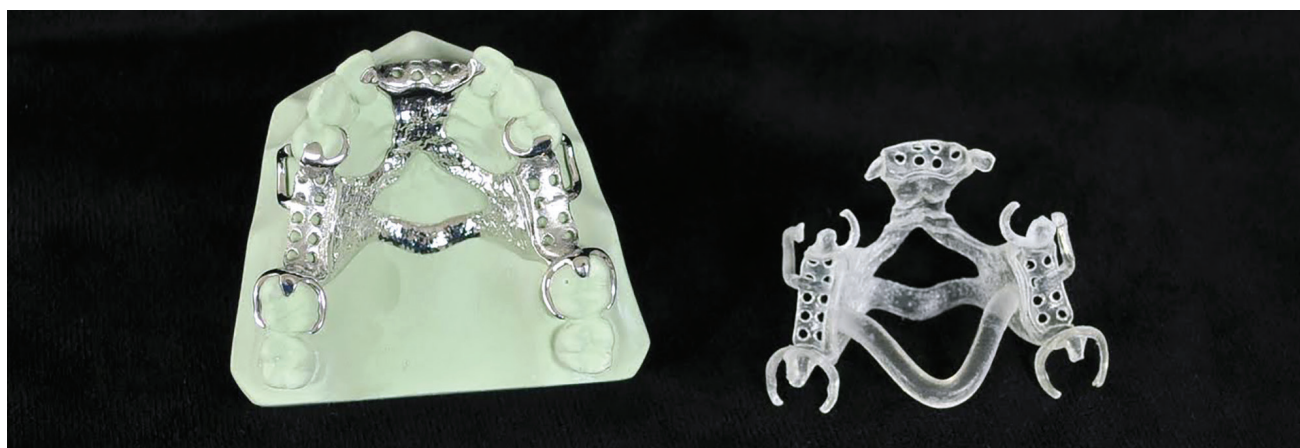
This cast frames, left, was created with the help of 3D printed biocompatible (MED610) material, right.
