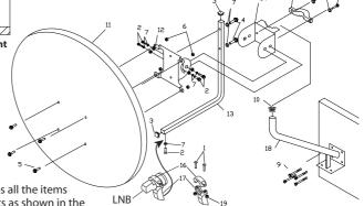
**4) Mount the Wall Bracket:** Mount the wall bracket (18) using the expansion bolts (9). Make sure that the mounting holes are drilled into brick or stone and not into the mortar. Also ensure that the wall mount is horizontal and perfectly level (check using a spirit level).
