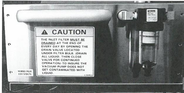
**DAILY:** Drain all moisture from the filter enclosure. Turn the drain knob counter clockwise to drain.
