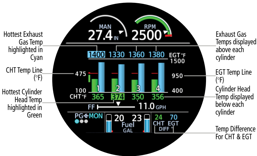
CHT/EGT - Four Cylinders - Bar Graph Example
