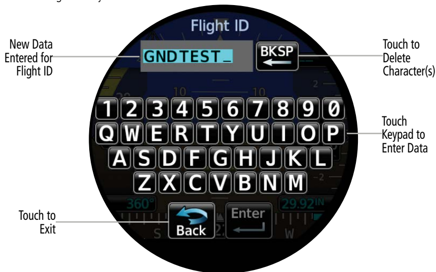
Flight ID Keypad Entry
