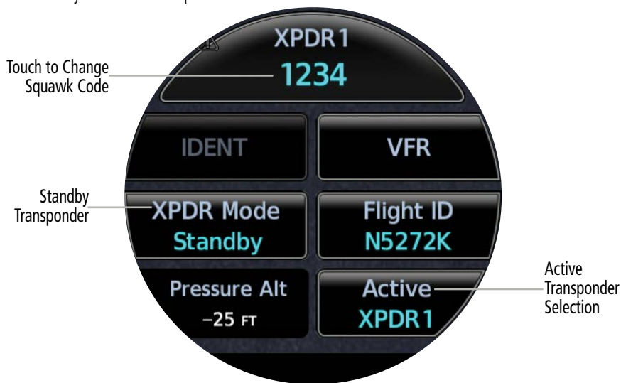
ADI - Transponder Control Display - Change Squawk Code
