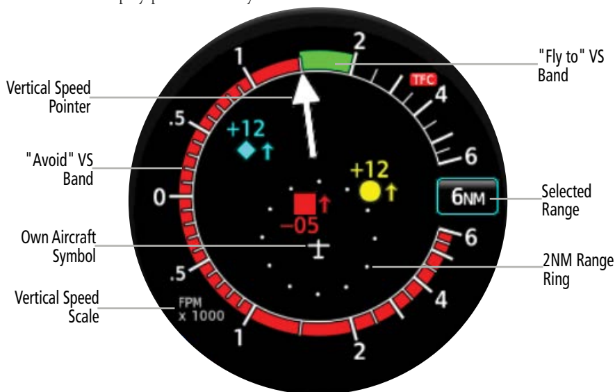
Instantaneous Vertical Speed Indicator
