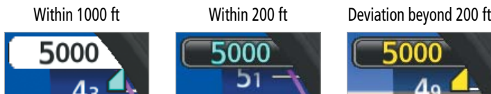
Altitude Alerting Visual Annunciations
