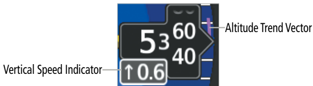
Vertical Speed Indicator and Altitude Trend Vector
