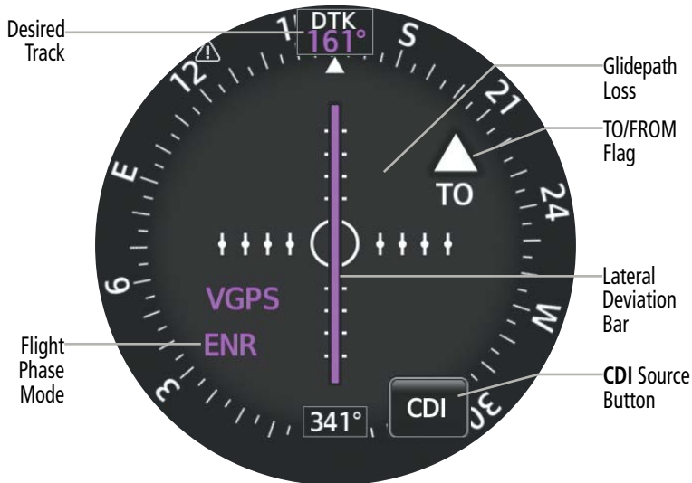
Typical 'CDI' Page with External GPS Navigator
