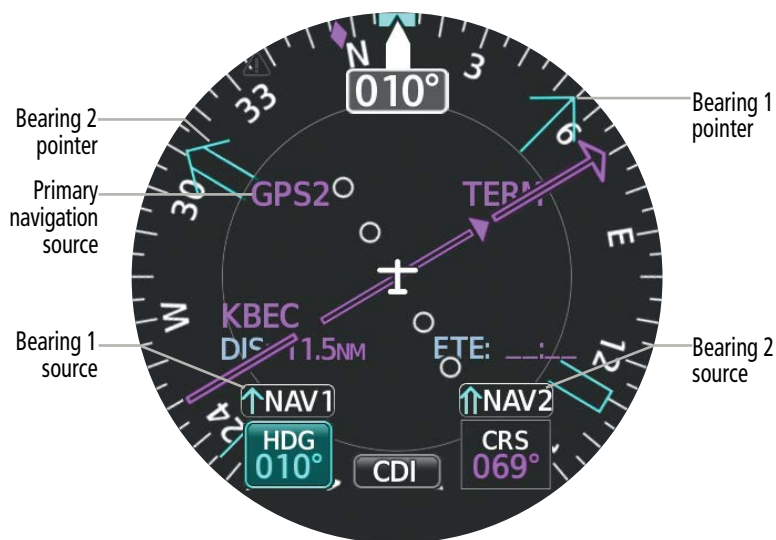
'HSI' Page with Bearing Pointers
