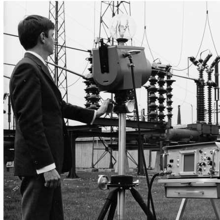
Figure 33.2 1969: ThermoVision Model 661. The camera weighed approximately 25 kg (55 lb.), the oscilloscope 20 kg (44 lb.), and the tripod 15 kg (33 lb.). The operator also needed a 220 VAC generator set, and a 10 L (2.6 US gallon) jar with liquid nitrogen. To the left of the oscilloscope the Polaroid attachment (6 kg/13 lb.) can be seen.
