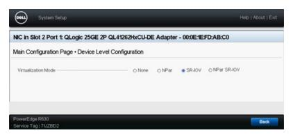
Figure 12-2. System Setup for SR-IOV: Device Level Configuration
