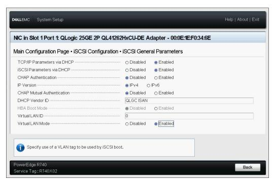
Figure 6-14. System Setup: iSCSI General Parameters
