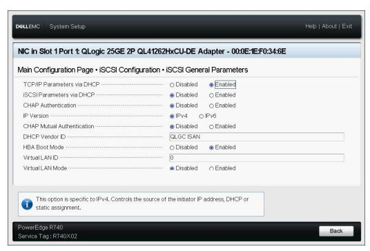
Figure 6-7. System Setup: iSCSI General Parameters
