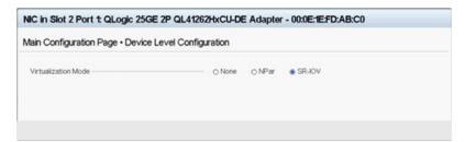
Figure 12-9. System Setup for SR-IOV: Integrated Devices
