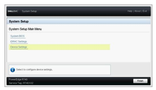
Figure 6-26. System Setup: Selecting Device Settings
