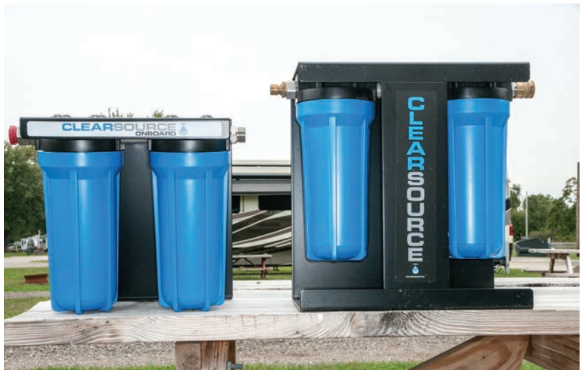
The onboard filter system (left) is quite a bit smaller and lighter than the external model. It's designed to be mounted in a utility compartment. It should not be installed in a storage compartment because of possible water leakage from burst hoses or worn gaskets.
