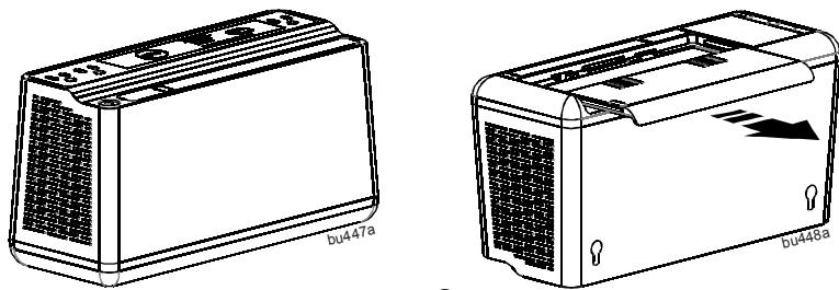
1 Remove the "Stop! Connect the Battery" label that covers the outlets. 2 Press the battery compartment cover release tabs located on the underside of the unit. Slide the battery cover off.
