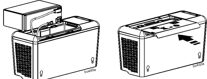
3 Connect the battery cable securely to the battery terminal. It is normal for small sparks to be seen when the battery cable is connected to the battery terminal. 4 Reinstall the battery compartment cover. Be sure that the release tabs lock into place.
