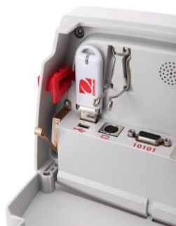
Interface connections inside of the Terminal.
