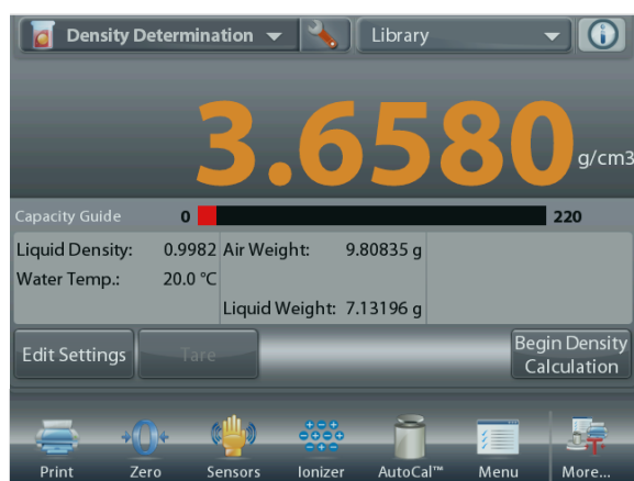
The DENSITY DETERMINATION – LIQUID Home screen
