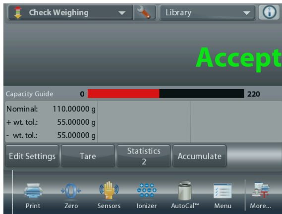
CHECK WEIGHING – Nominal/Wt Tolerance home screen
