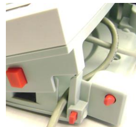
Interface connections inside of the Terminal.
