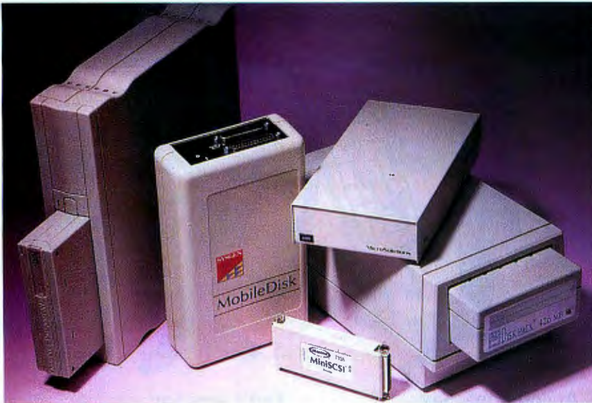
Photo 4: A collection of alternative drives. Removable hard drives best answer security requirements, but you won't want to ship them from place to place. Parallel-port-based drives are suitable for moving large files among machines or increasing the storage capacity of portable computers.
