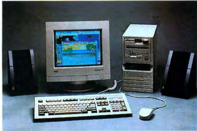
Clover Computer Systems' MPC-I has real-time window manipulation and a chroma key for overlaying finished live images on a VGA screen.
