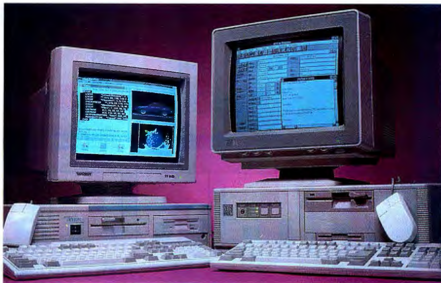
Tandon's Option 386SLC/50 (left) and Zeos's 486SLC-25 are the first desktop systems to include Cyrix's 486-compatible Cx486SLC.
