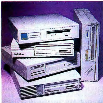
Photo 3: Removable drives come in many shapes and sizes besides MO drives. The SyDOS and Microtech drives provide removable hard disk platters. The Procom floptical drive, in addition to supporting 21-MB floptical disks, can also read and write standard 720-KB and 1.44-MB floppy disks. The Bernoulli drive provides high-speed access using sturdy 90-MB cartridges.
