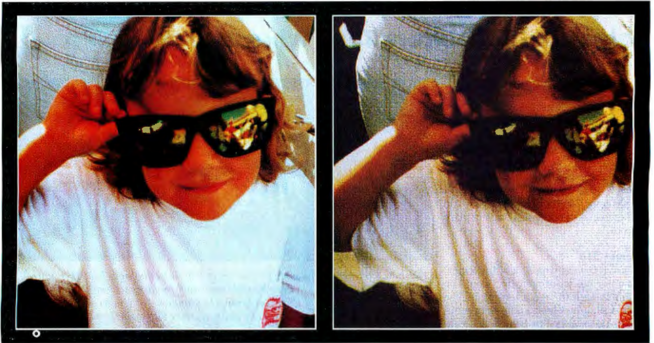
The Canon CJ10 output (left) is sharp and clear; the special Canon paper makes the colors virtually leap off the page. The HP XL300 output (right) doesn't have the banding problem of the CJ10, but its colors tend to be a bit murky compared to those of the Canon output.
