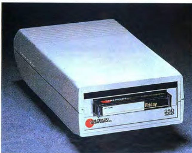
The plug-and-play Trakker tape backup device supports the enhanced PC parallel port.
