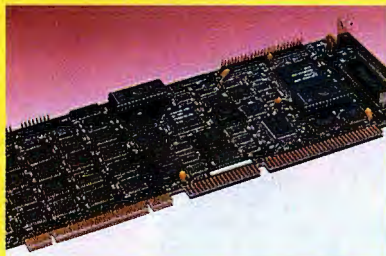
Photo A: The Micronics VL-Bus motherboard shows a typical layout for the local bus slots. The VL-Bus extensions appear adjacent to the upper two ISA slots.
