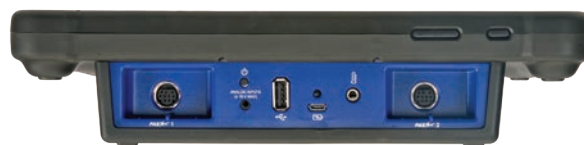
The SPARK LXi features two PASPORT ports as well as ports for the included temperature and voltage probes.
