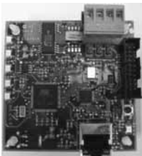
BACnet® COMMUNICATION CARD RXXR-AY01
