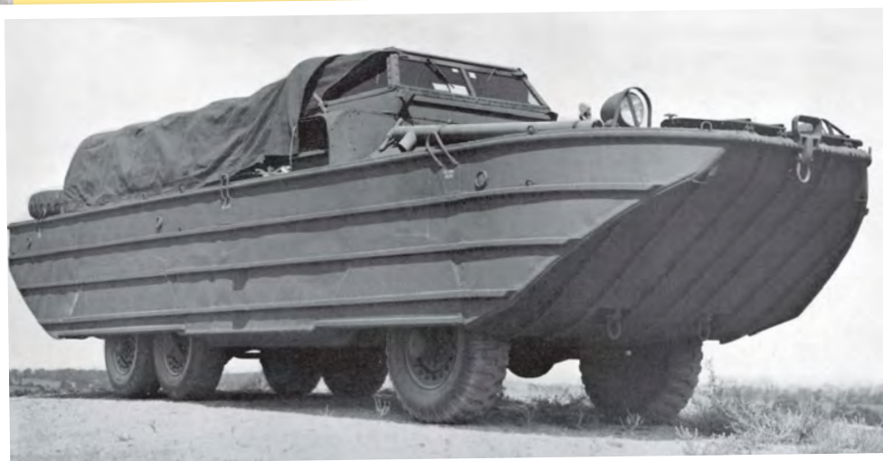
Production DUKW with the later windscreen in which the sides were angled rather than straight; this vehicle lacks the central tyre inflation system (CTIS) that was fitted from early 1943.
