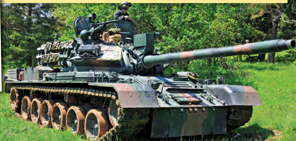
Below: Based partly on the Russian T-55 the TR-85 M1 Bizonul main battle tank is fitted with the 100mm A308 rifled tank gun, a coaxial 7.62mm PK general purpose machine gun, a 12.7mm DShK heavy machine gun and a smoke grenade discharger system with 20 launch tubes. The MBT has a gross vehicle weight of 50,000kg, is 9,920mm long, 3,430mm wide and 2380mm high.
