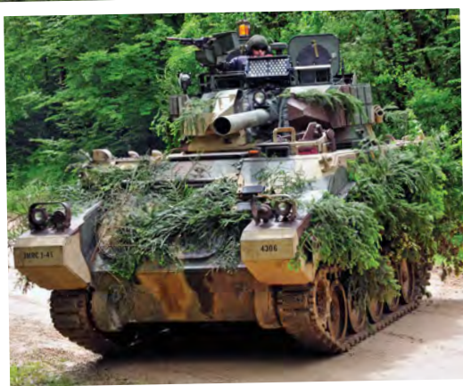
Above: The Tank Company of the 1st Battalion, 4th Infantry Regiment, the in-house OPFOR of the JMRC, uses the M113 based OPFOR Surrogate Vehicle – Tank (OSV-T). The OSV-T is used to act as a T-80 MBT and its MILES equipment simulates the effects of a 125mm tank gun.
