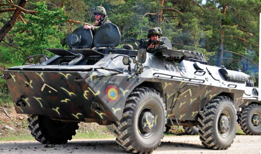
The mortar platoon of the Romanian Armoured Battle Group fielded a couple of TAB-79AR mortar carriers. The amphibious 4x4 driven wheeled armored vehicle is fitted with an 82mm M-1983 mortar. The mortar can be fired from the vehicle or used in a dismounted role.
