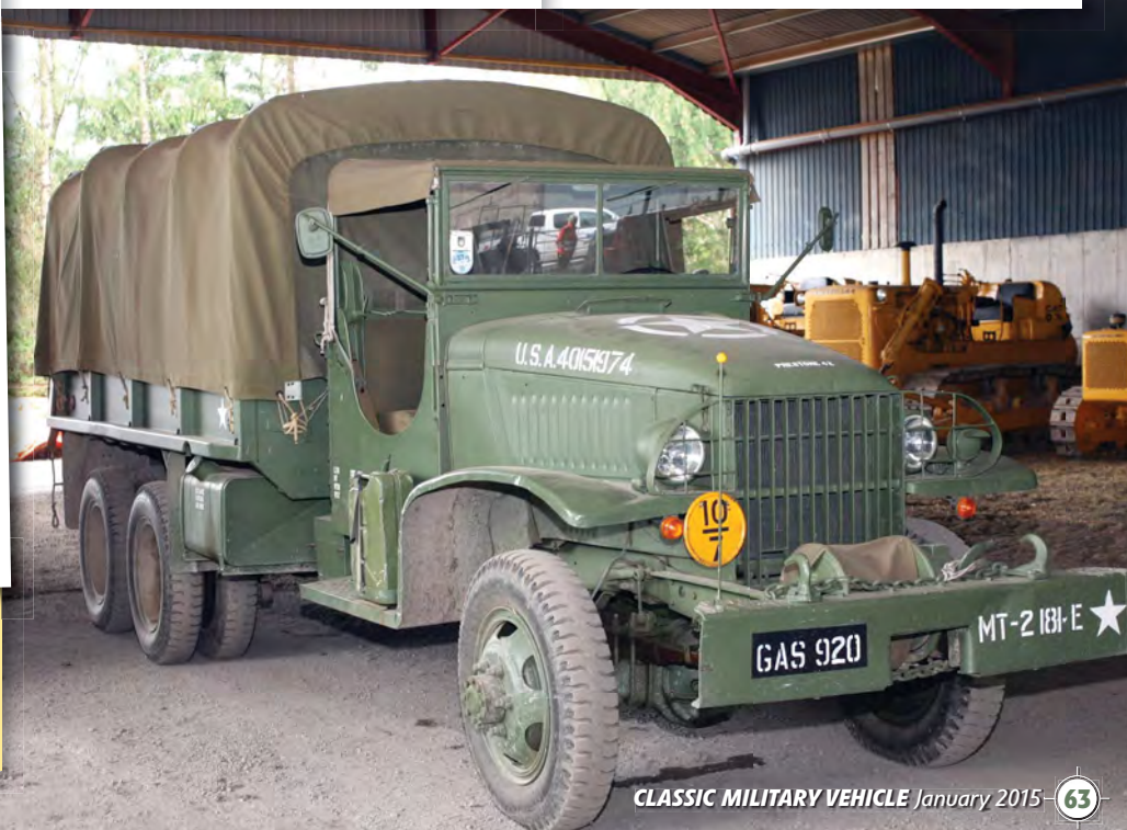
Above: GMC 353 was equipped with fold-up troop benches along each side of the interior. Right: GMC 353 general cargo truck had been converted to run on LPG – the hammer fell at £5000.
