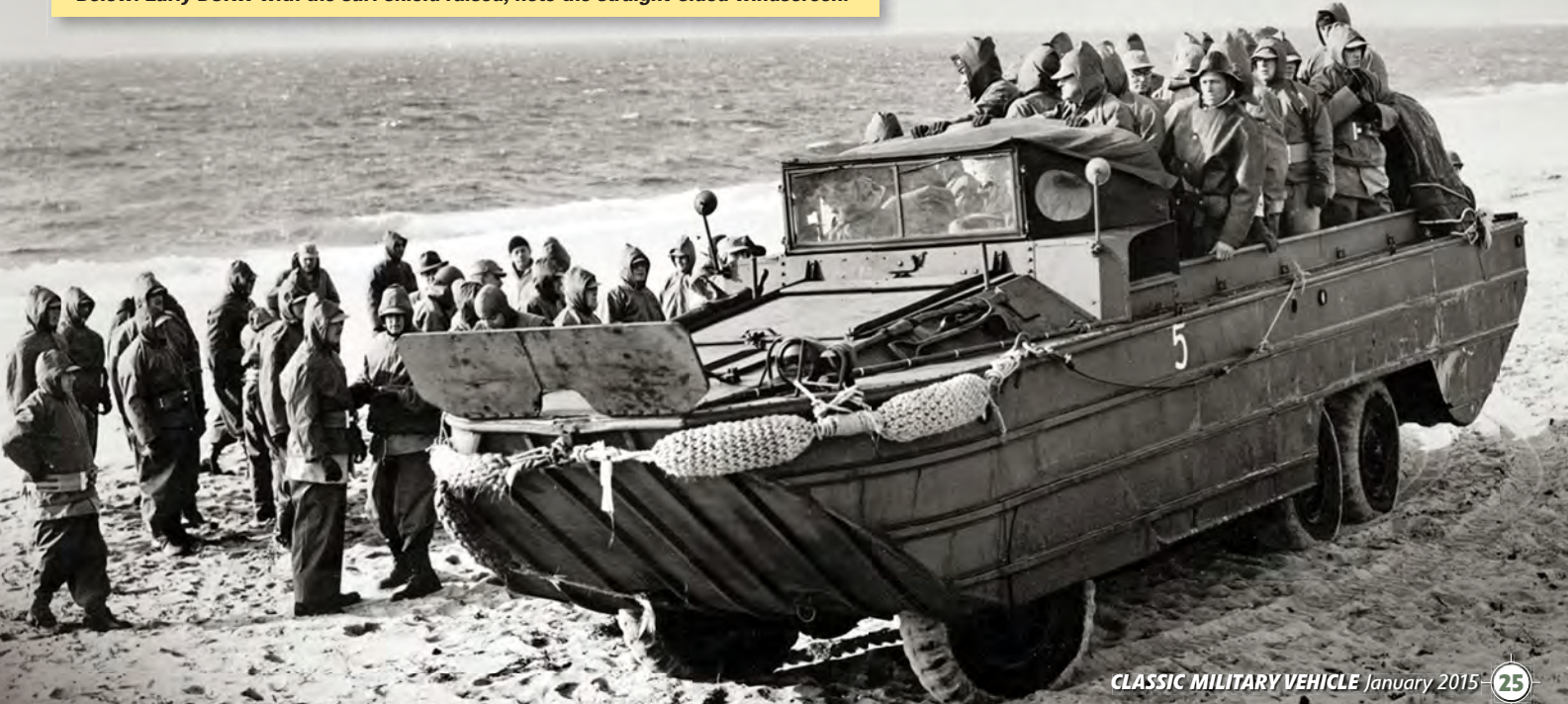
Below: Early DUKW with the surf shield raised; note the straight-sided windscreen.
