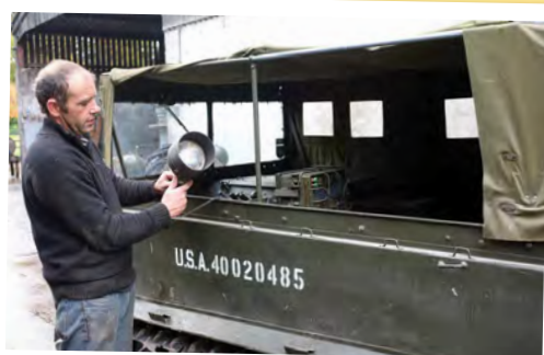
Above: Maintenance engineer Dave Gurney, demonstrates the Weasel's detachable spotlight.
