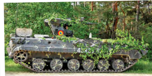
The armoured infantry company of the Romanian Armoured Battle Group fielded MLI-84M 'Jderul' armoured infantry fighting vehicles. The Romania-built variant of the Russian BMP 1 is fitted with an OWS 25R stabilized overhead weapon station that features a 25mm automatic cannon, a coaxial 7.62mm machine gun and a Spike anti-tank guided missile launcher.
