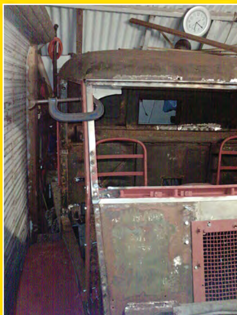
A second cab was sourced from the Muckleburgh Collection. It had a bad case of tin worm but elements were salvageable. (Daniel Smith)
