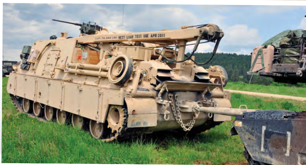
The US forces use the M88 A2 Heavy Equipment Recovery Combat Utility Lift and Evacuation System (HERCULES) as armoured recovery vehicle. Here the vehicle is towing an M1 A2 SEP (V2) Abrams main battle tank.
