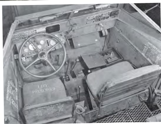
Above: Interior of the driving position showing the major controls; the box on the floor ahead of the passenger seat controls a rocket-launcher system.
