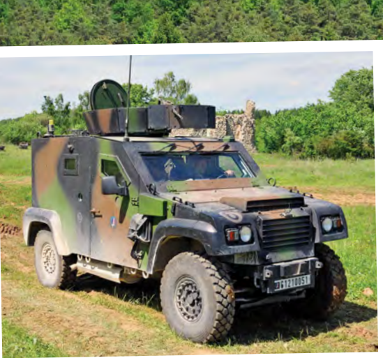
Above: For command and liaison purposes the French troops employed a couple of Petit Véhicule Protégé (PVP). The light armoured 4x4 PVP is 4.6m long, 2.28m wide, 2.17m high and has a combat weight of 4.4 tons. The vehicle can be armed with a 7.62mm machine gun, as seen here, or a 12.7mm heavy machine gun.
