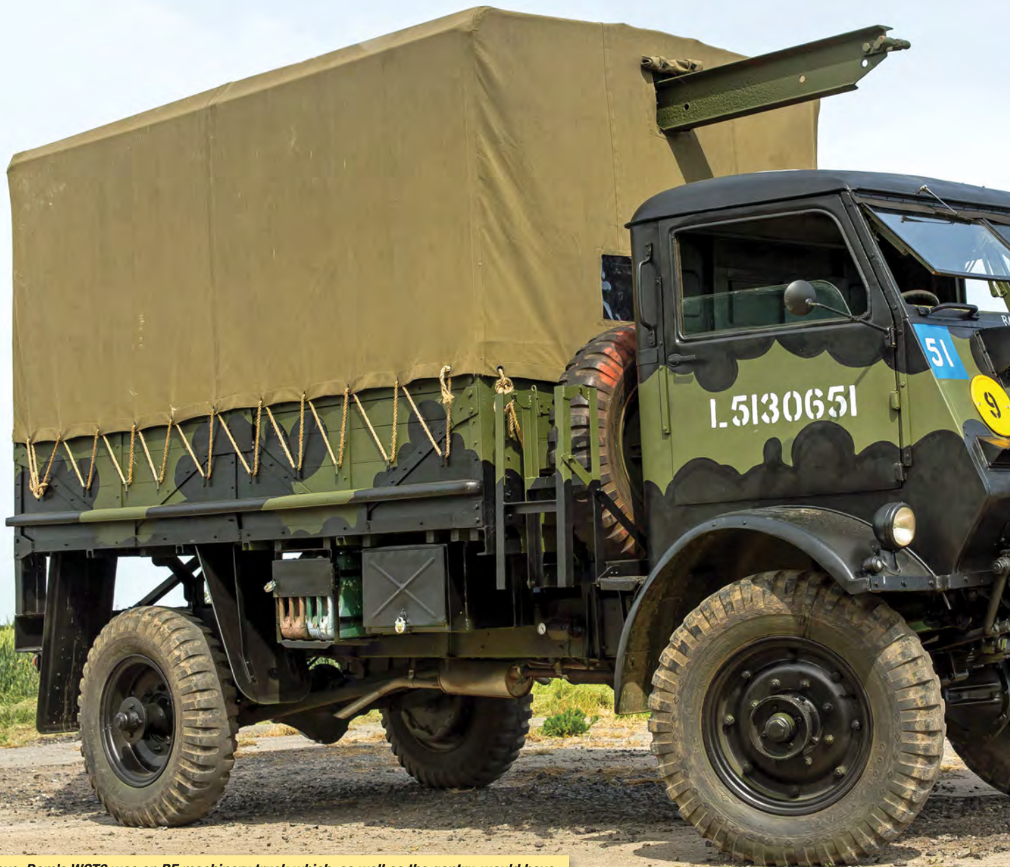
Above: Dom's WOT6 was an RE machinery truck which, as well as the gantry, would have been equipped with a 24Kw generator and a variety of tools.
