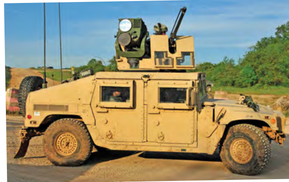
The Scout Platoon of the 2nd Battalion, 5th Cavalry Regiment employed a mix of M3A3 Bradley cavalry fighting vehicles and M1151A1 HMMWV Expanded Capacity Armament Carrier IAP/Armor Ready fitted with the Long Range Scout Surveillance System (LRAS3).
