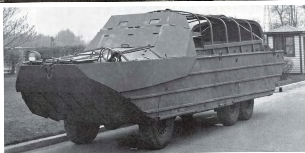
DUKW fitted with experimental frontal armour intended to be supplied as a kit for use in the field. Constructed from face-hardened steel, the forward-facing plates were 9.5mm in thickness, whilst those at the side were 6.5mm.
