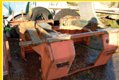
The panels of the cab that originally came with the WOT6, seen here inverted, had been welded together. (Daniel Smith)
