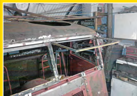
Above and left: Unfortunately, few photos exist of the restoration process; these two showing the windscreen frame and surrounding area – which had been badly affected by rust – give a small indication of the effort and skill that Dom put into the project. (Daniel Smith)
