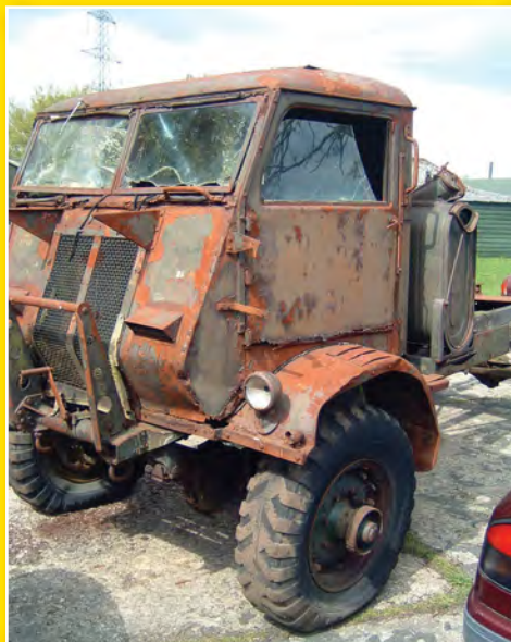
A second cab was sourced from the Muckleburgh Collection. It had a bad case of tin worm but elements were salvageable. (Daniel Smith)
