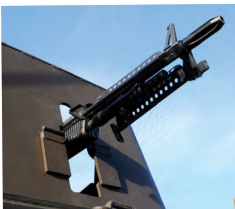
Gun shields were improved early on to address high crew casualty rates.
