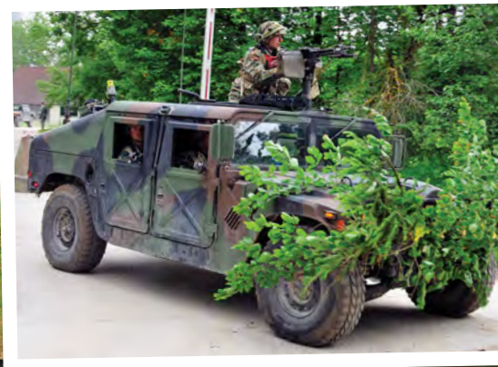
Below: A couple of nations that took part in exercise Combined Resolve deployed their troops without vehicles and borrowed US vehicles for the duration of the exercise. Here Bulgarian infantry can be seen operating a US Army M1025 HMMWV Armament Carrier with Basic Armor.
