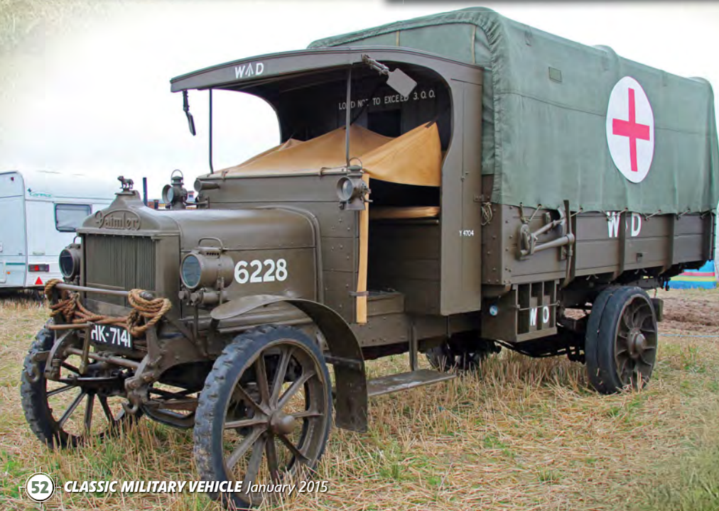
Below: This 1915 Daimler Y Type dates from 1915 and was built at the AEC factory in Southall. It had a top speed of 20mph (32km/h) and is powered by a four-cylinder petrol engine. Little is known of its activities during the Great War but when it was purchased by current owner Ronald Harris it was still in its original wartime livery.
