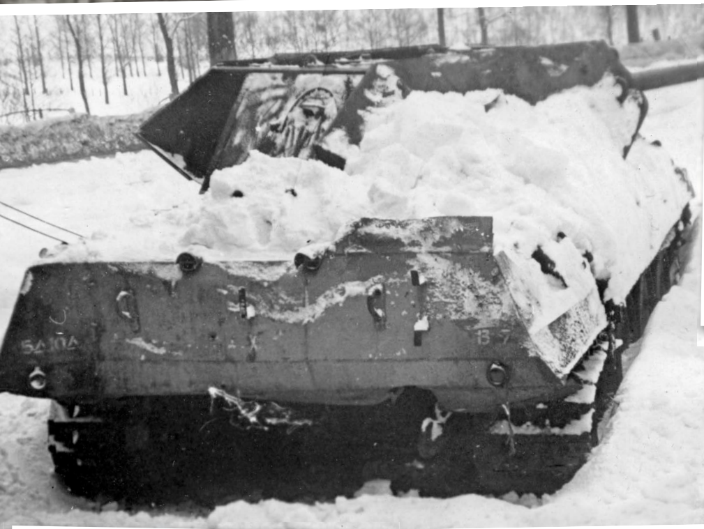
Above: A rear view. Note the dummy brackets and fittings and the ports for the Panther's exhaust. Left: A close-up showing the false gun shield and turret sides complete with dummy studs and lifting rings.
