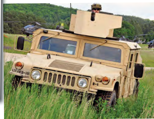
An M1151A1 HMMWV Expanded Capacity Armament Carrier IAP/Armor Ready provides security for the airfield of the aviation assets of the US-led multinational NATO contingency force. The vehicle is fitted with a Gunner Protection Kit.
