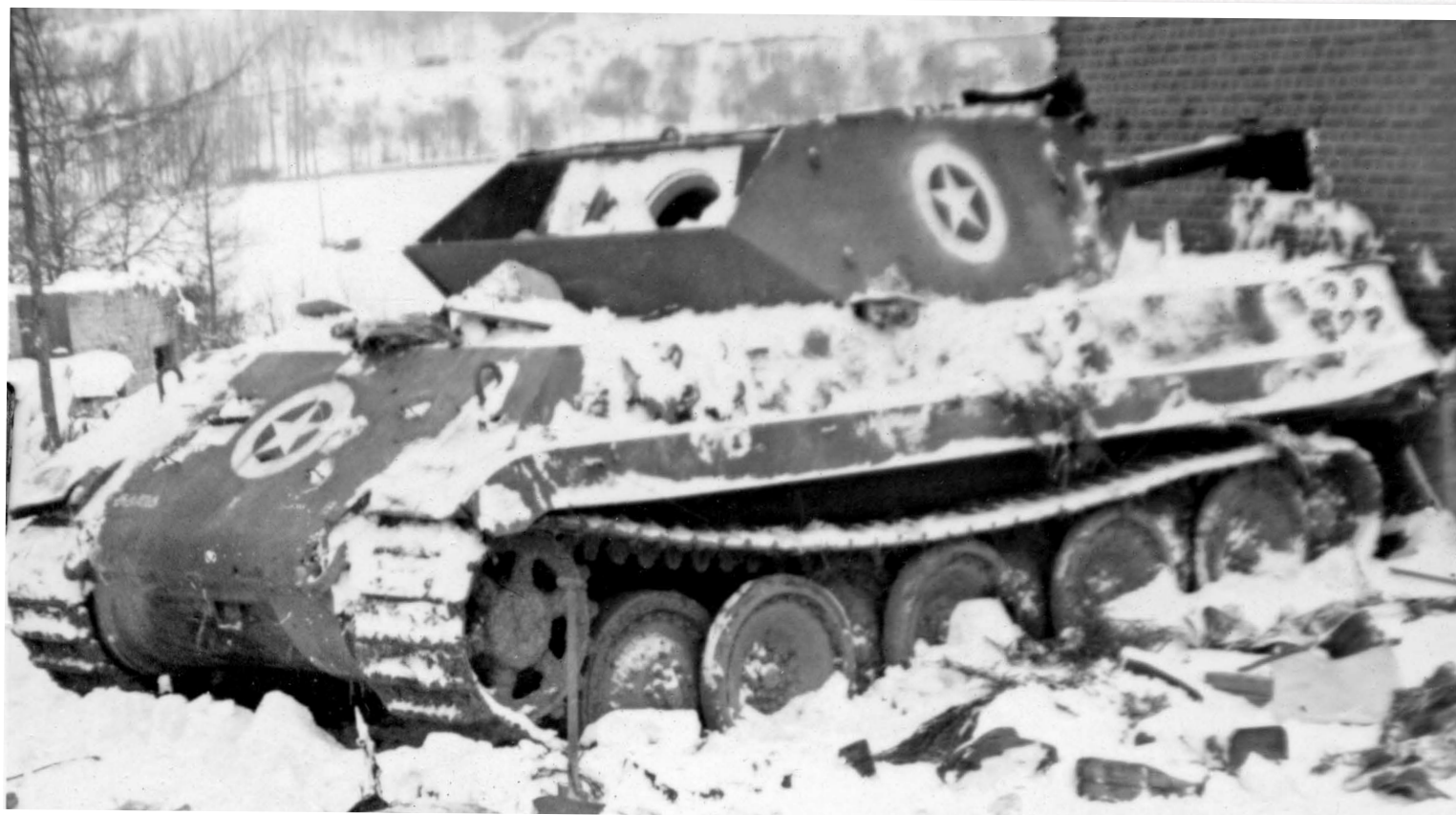
Above: A left front view with the turret reversed. Note the false final-drive housings and side apron. Left: Wheels and tracks aside, the fake M10s are very convincing. Note the rectangular aperture on the false front to allow the use of the Panther's bow machine gun. Bottom left: A wartime photo of Otto Skorzeny, complete with duelling scar.
