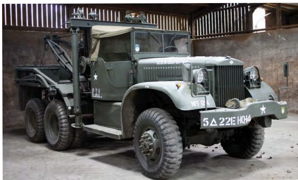
Holmes equipment, two 5-ton winches at the rear and a front mounted winch. The canvas topped cab would date this vehicle to post 1943, so technically it's a 969A. Lastly we come to what for many will be one of the ultimate WW2 military vehicles,
