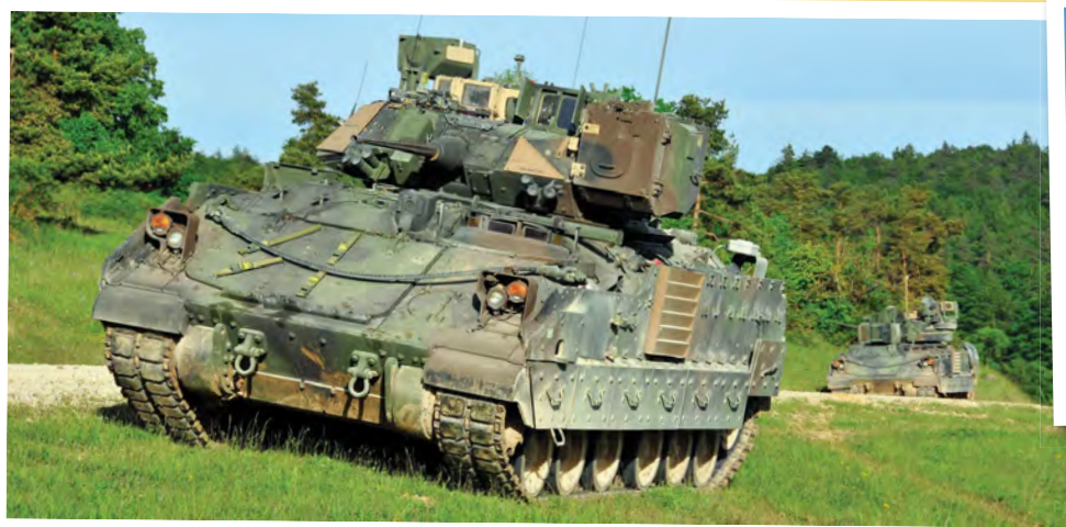
Instead of a TOW launcher the Bradley Fire Support Team Vehicle (BFIST) is fitted with the Fire Support Sensor System (FS3). The vehicle is used by fire support teams to direct mortar and artillery fire. The FS3 is a long-range multisensor system that allows to detect, recognize, identify and geo-locate targets in real time.
