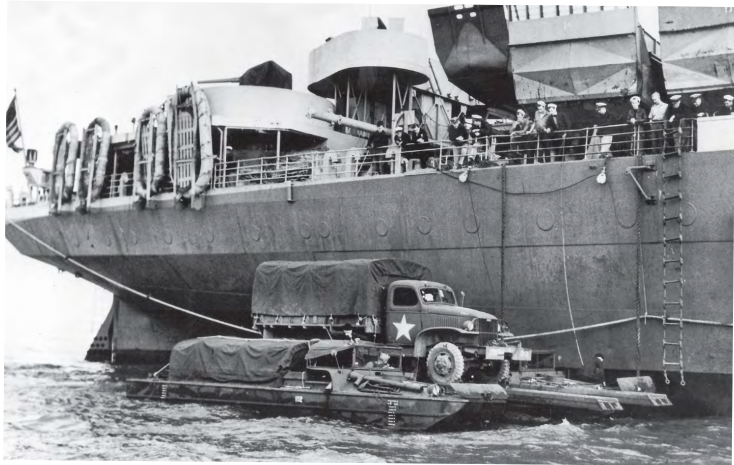
Dry ferry in use carrying a GMC 2.5-ton 6x6 truck. The treadways which were used to support the truck were 31ft (9.455m) long and the ferry could support a load of 65,000 lb (29,545kg) which was sufficient to allow a Sherman tank to be transported in this way.
