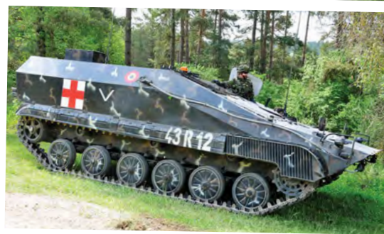
Above: The MLI-84M Vehicul de Evacuare Medicală is the armoured ambulance version of the MLI-84M AIFV. The hull of the vehicle features a raised roof. The vehicle can carry four patients on stretchers and carries a wide range of medical equipment.
