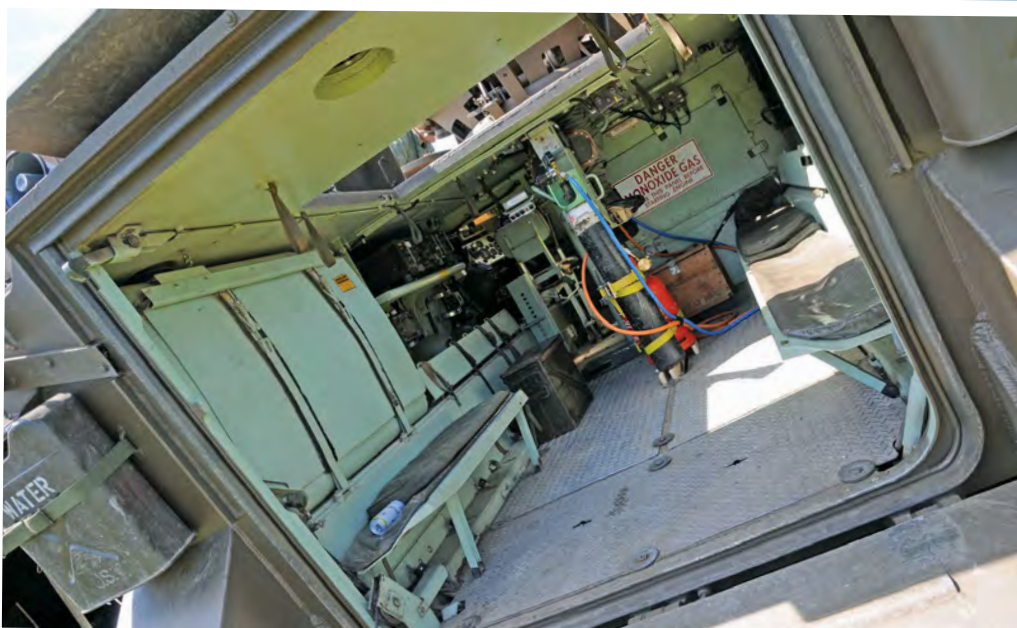
Rear exit port allowed quick troop dispersion. Crews sat on benches facing inwards.
