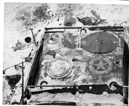
Above: A top view of the turret showing the hatch covers used in lieu of the Panther's cupola. Right: The plate over the machine-gun aperture is visible to the left of the star. Although partly hidden by the gun barrel you can just make out an aperture for the Panther's coaxial machine gun.
