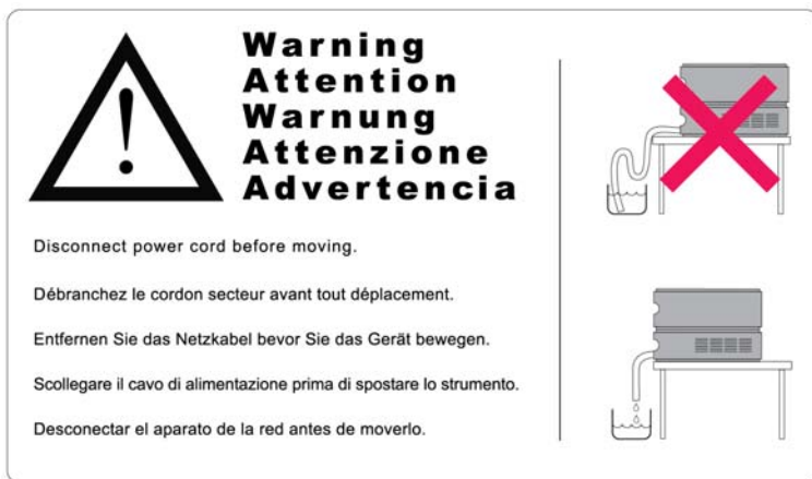
Figure 8 Warning label (illustration for correct waste tubing)
