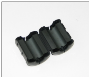
Figure 2-4 Clamp-on EMI Filter (Open)
