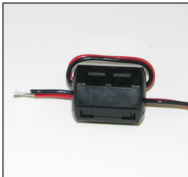
Figure 2-6 EMI Filter Installed
