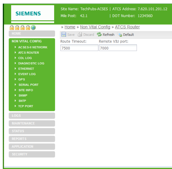
Figure 7-20 ATCS Router Configuration Screen
