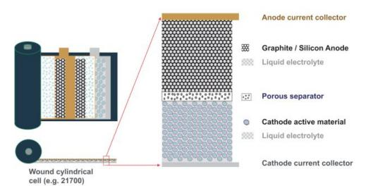
The energy density of conventional lithium-ion batteries is fundamentally limited by the anode, which provides a host material to hold the lithium ions, preventing them from binding together into pure metallic lithium. Metallic lithium, when used with conventional liquid electrolytes and porous separators, can form needle-like crystals of lithium known as dendrites, which can penetrate through the separator and short-circuit the cell.
