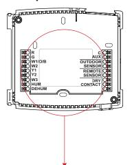
To remove the thermostat backplate: Gently separate the display from the base by pulling first from one side, then the other until the two pieces unsnap. A small screwdriver may be used, very carefully, to start seperating the two pieces.
