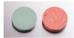
Fig. 27: Superior mixing quality of Express™ 2 Penta™ Putty with the Pentamix™ Mixing Unit (left) compared with a putty mixed by hand (right, Express™ STD Putty).
