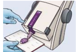
Fig. 32c: Material extrusion until mix is homogeneous.
