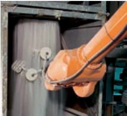
More output, less down-time: robot-based automation optimizes ceramic shell making.
