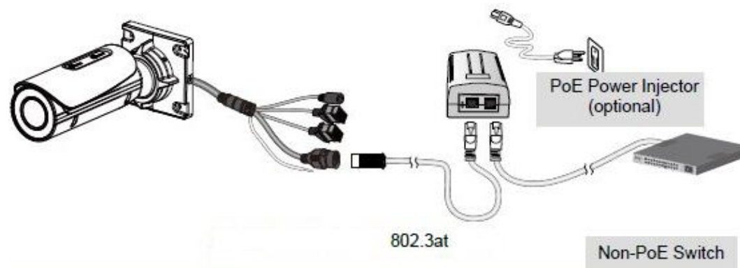
Figure 1-3 Connecting the Camera to a Non-PoE Switch
