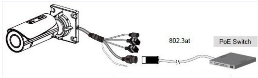
Figure 1-2 Connecting the Camera to a PoE-Enabled Switch
